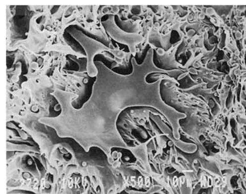
Figure 5 Micrographs of fractured surfaces of tested type I noncompatibilized (NC) specimens containing a weldline (perpendicular to flow view). (A) skin; (B) and (C) core.
